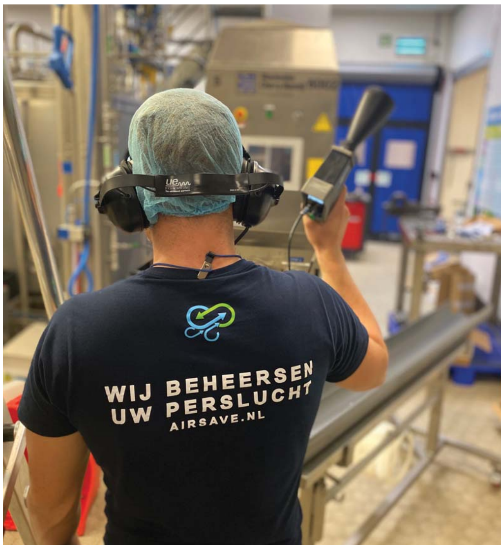
Airsave uses a noise detection system to identify compressed air leaks; a filter system enables operators to work in noisy environments.
